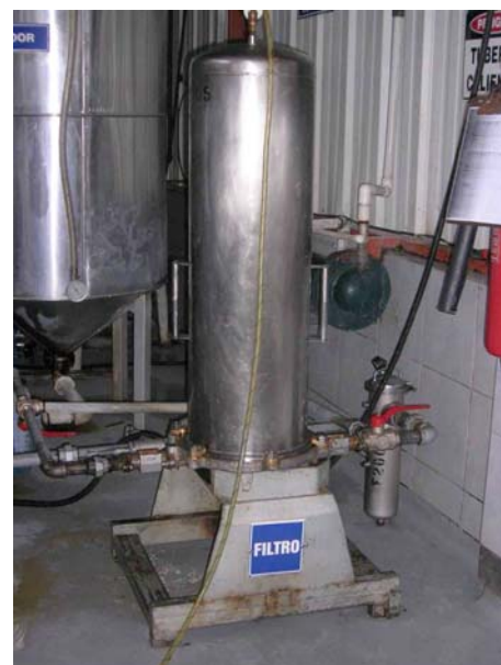
Pic 10: Filter final stage before entering the storage and pumping filling stations
