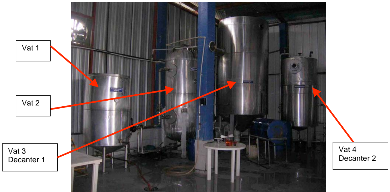
Pic 6: The liquid is now ready to go to the fish oil production plant.
