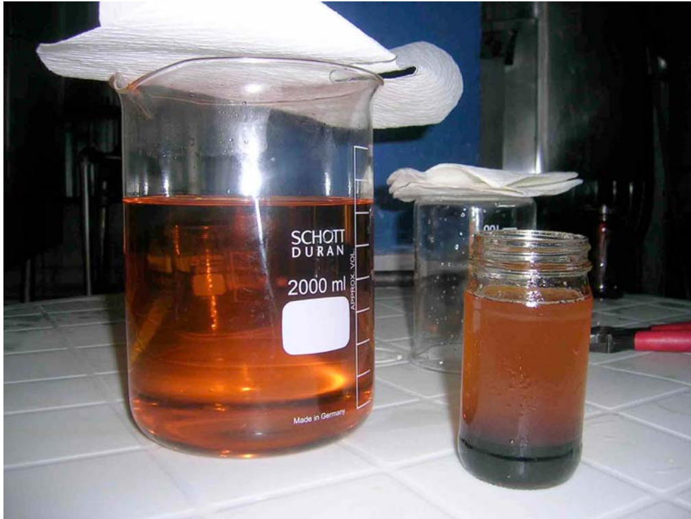
Pic 8: Cleaned and purified oil to the left and un-cleaned and dirty (containing glycerine in bottom) oil on the right.
