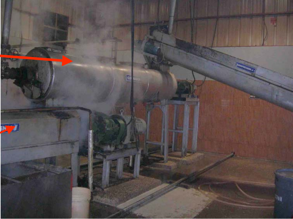
Pic 4: Expeller: Separates liquid from biomass
