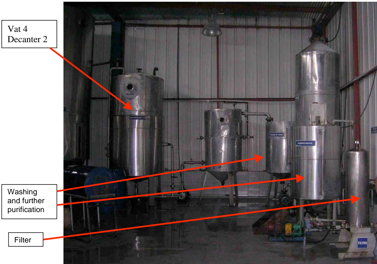
Pic 9: Washing of the bio-diesel and further purification
