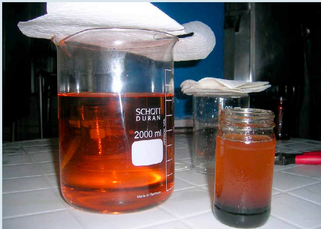
It is possible to produce about one litre of biodiesel from one kilogram of fish slaughter waste.
